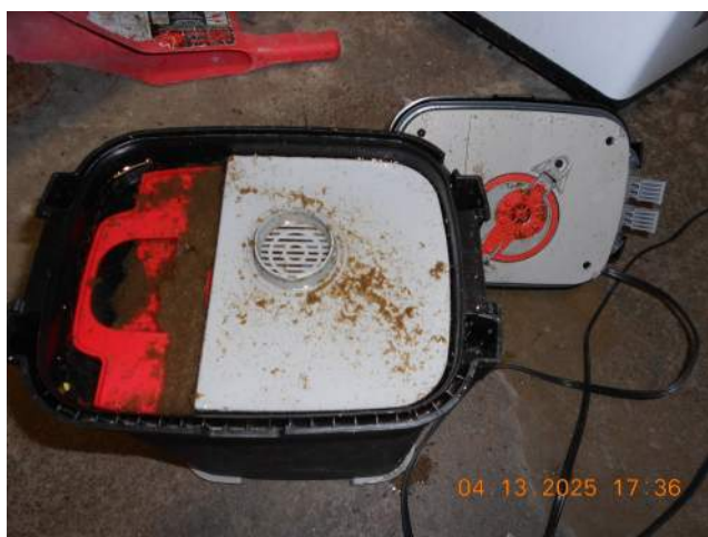
What you find when you open a filthy 307. Sponges on the left, filter baskets under the gray cover on the right. Lid on the floor with impeller visible.
